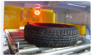
The principle of operation of the device is to determine the overall dimensions of the tires moving on the roller through the supplied device with a light measuring system. The tire stops and centers in a specific location using two gate flaps to determine the type of tread by the technical vision camera.
